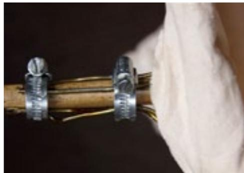
7. Wrap the wire and jubilee clips in duct tape to cover all sharp edges and you have finished making your sweep net.
