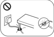
Do not operate this unit if the cord or plug is damaged.
