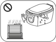
Do not operate the unit next to heat sources such as radiators.
