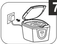
When cleaning is finished, unplug the unit from the mains and open the lid to remove the item. Pour away the water and wipe the stainless steel tank with a clean dry cloth.
