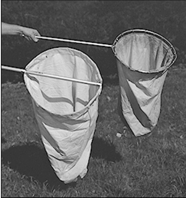
Figure 9: Two sweep nets. The one above is rather shallow and not very wide. The one below is a useful size, has a strengthening bar and it is deep enough so that active insects will not escape too easily
