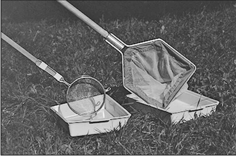
Figure 23: A simple water bug catcher made by taping a kitchen sieve to a length of wood and a professional pond net
