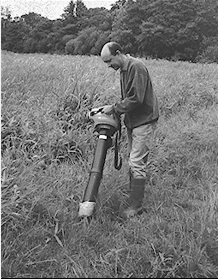
Figure 21: Suction sampling using a modified garden blow-vac.
