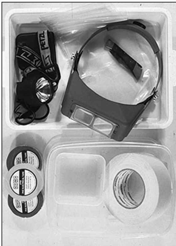
Figure 6: Other useful bits of kit (PVC tape, gaffer tape, tupperware™ boxes, sorting tray, head-torch, strong lock knife, zip-lock plastic bags, head-band magnifier)
